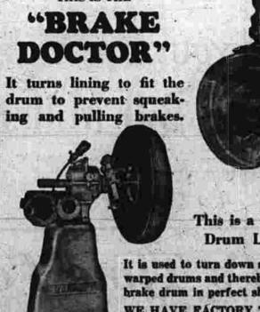
It is used to turn down scored and warped drums and thereby puts the brake drum in perfect shape. WE HAVE FACTORY TRAINED MECHANICS TO OPERATE THESE MACHINES
